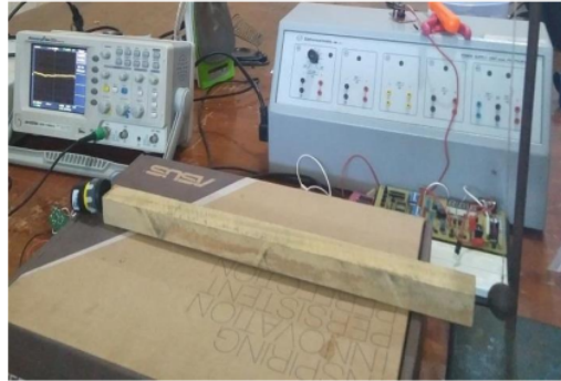
Figure 2. Testing of acoustic properties with oscilloscope screen
